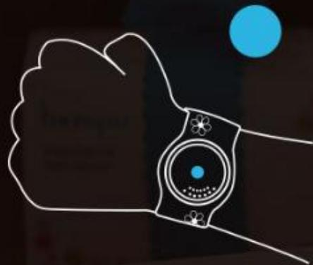
BEMPU flashes a blue light when the baby is at a normal temperature
